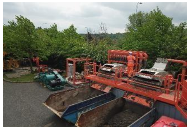
Fig. 5: Image taken of the mud treatment and shaker
