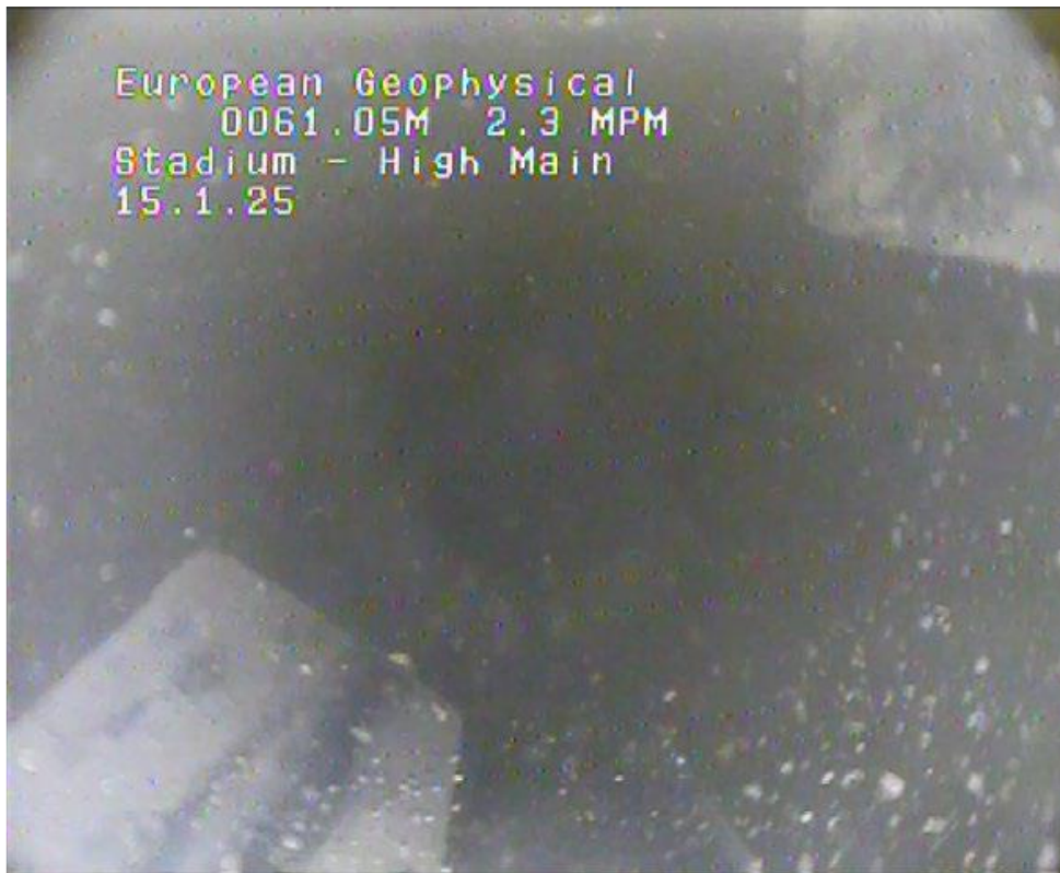
Figure 2: Slipped 'grout basket' at the base of the casing at Stadium High Main borehole.
